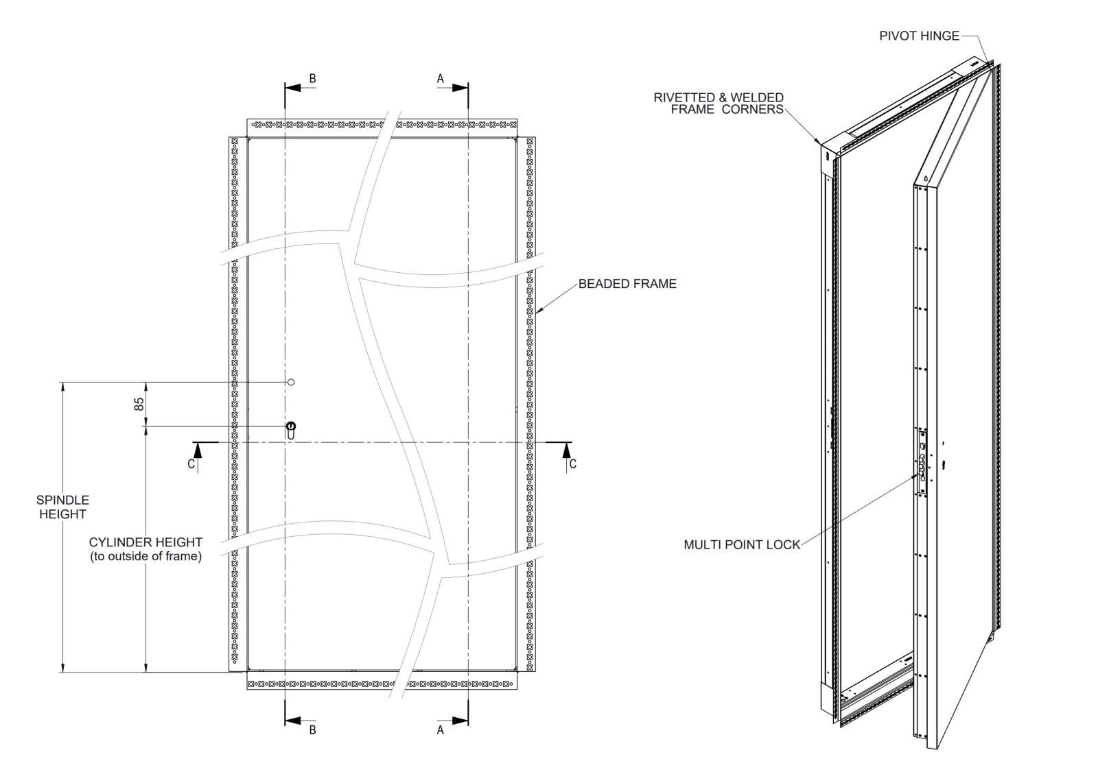
Panel size normally measured to outside faces of frame (e.g. A mm x B mm) Recommended Prepared opening 5 to 10mm greater than panel size (e.g. A+10 mm x B+10 mm) Beaded frame panel finish primed powder coat white, Picture frame panel finish RAL 9010 gloss white.
