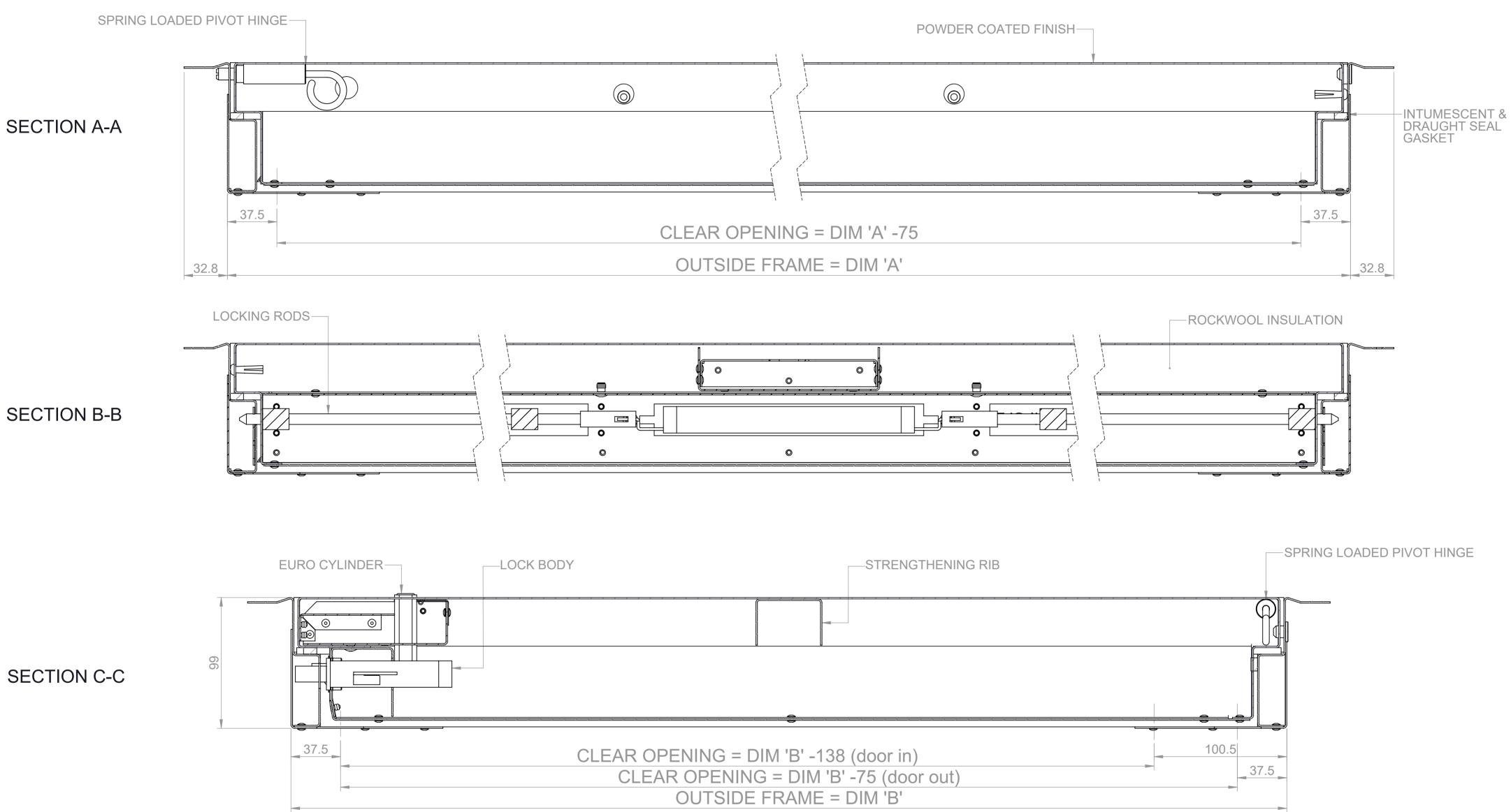
Panel size normally measured to outside faces of frame (e.g. A mm x B mm) Recommended Prepared opening 5 to 10mm greater than panel size (e.g. A+10 mm x B+10 mm) Beaded frame panel finish primed powder coat white, Picture frame panel finish RAL 9010 gloss white.
